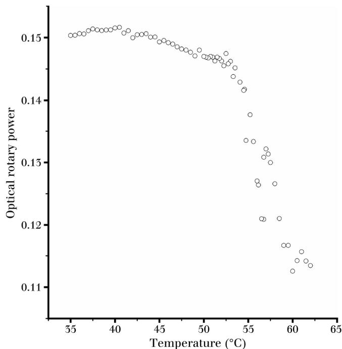
**Figure 5.** Variation of ORP ( $\text{deg } \mu\text{m}^{-1}$ ) with temperature in the SmC\* phase
