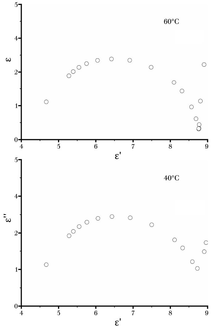
Figure 3. Representative Cole-Cole plots at at 60°C and 40°C
