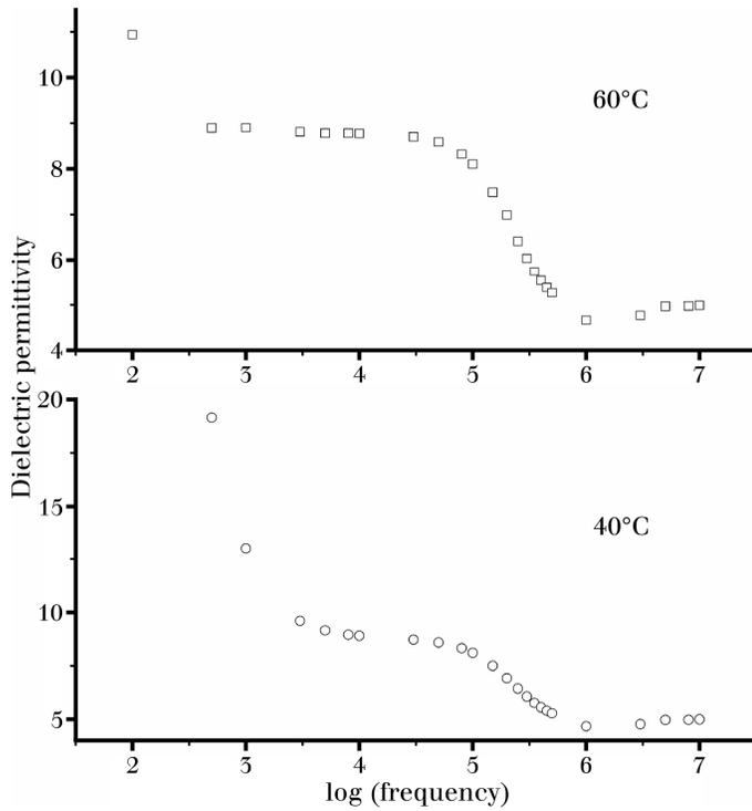
Figure 1. Variations in dielectric permittivity with the log of frequency (Hz) at 60°C and 40°C
